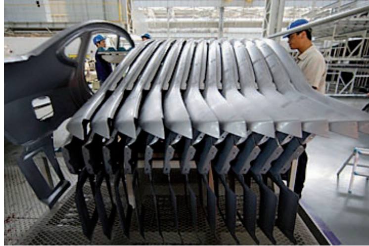
Figure 5: Pressed metal automobile (car) parts in the Hyundai car plant in Beijing
